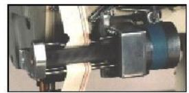
Mount the standard metering mechanism on top, bottom or side to feed elastic, tape or other narrow fabric up to 3" wide
